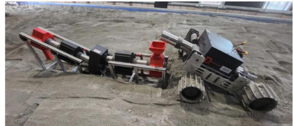
Figure 2: Excavation module attached on a rover collecting loose regolith and feeding another MDC
